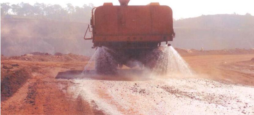
Dust suppression system by water sprinklers procured from BEML having capacity of 28000 litres.
